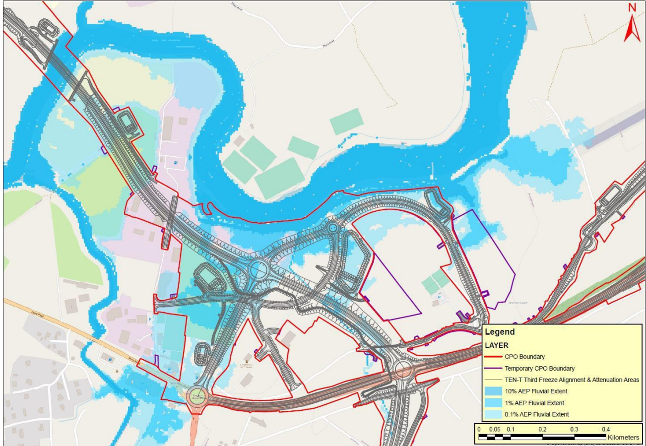
Figure 3.5 River Swilly Crossing - CFRAM current fluvial flood extents with proposed route alignment
