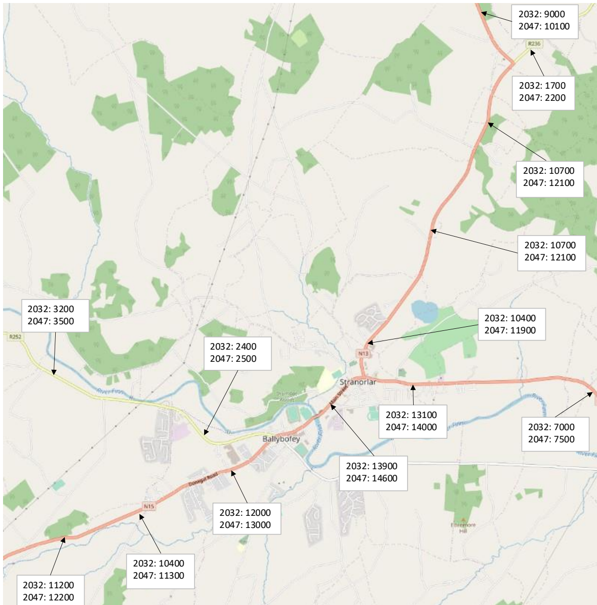
Figure 6-33 – Ballybofey/Stranorlar Do-minimum 2032 & 2047 Traffic Flows with A5 WTC
